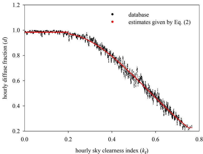
Fig. 1. Comparison of the  $d - k_t$  data with those predicted using the proposed model
